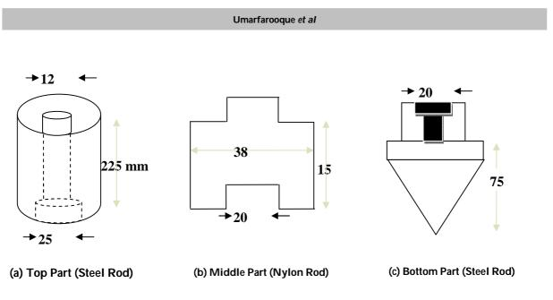
Fig.3. Schematic Diagram of Soil Moisture Sensor
